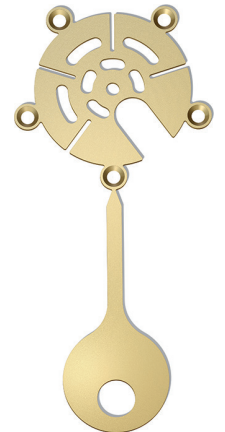
13-000091 micro shunt plate, Ø21 mm, 5-hole, T = 0.6 mm
